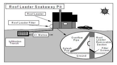
granular stone. Infiltration trenches are typically designed with a perforated pipe inlet intercepting water collected on a roof or pedestrian area. The design of Infiltration trenches depends on its purpose and site characteristics.
