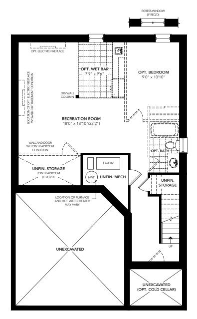
OPT. FINISHED BASEMENT FLOOR PLAN ELEVATION 'A' & 'C'
