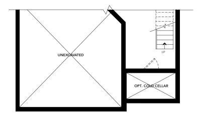
BASEMENT FLOOR PLAN ELEVATION 'B'
