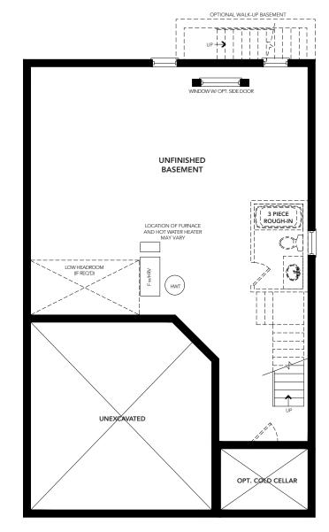
BASEMENT FLOOR PLAN ELEVATION 'A' & 'C'
