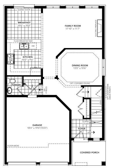
GROUND FLOOR PLAN ELEVATION 'A'
