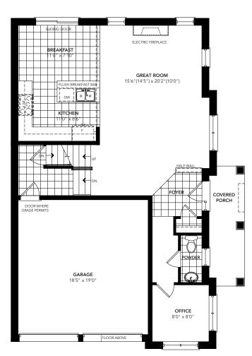
GROUND FLOOR PLAN ELEVATION 'B'
